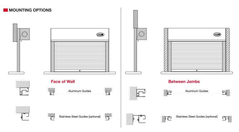
Standard counter shutters are built to order to fit specific dimensions up to 14'4" wide, 8'4" high. Consult factory for larger doors not listed. If headroom is critical, consult factory to determine headroom requirements for your application.
